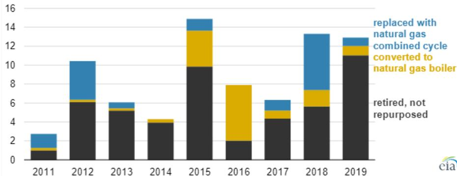
U.S. coal-to-natural gas plant conversions by conversion type and capacity (2011-2019)
